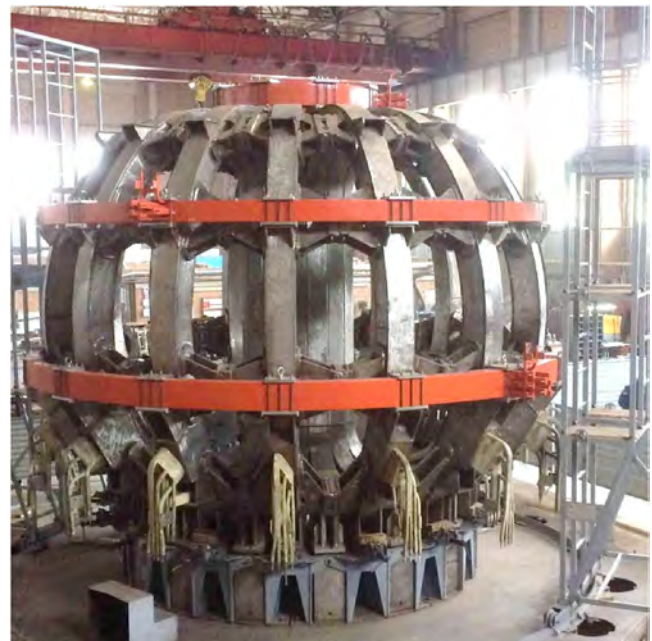
Fig. 9. Toroidal winding together with poloidal field coils.
