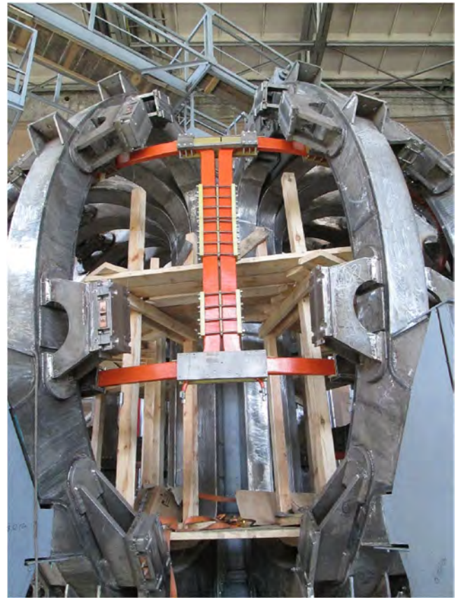
Fig. 8. Placements of HF coils inside toroidal winding.
