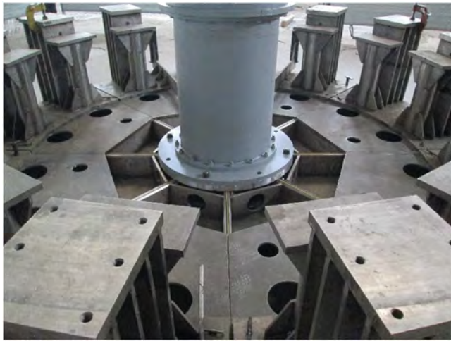
Fig. 6. Technological column and support structure.
